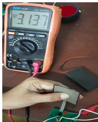
Fig. 3 (a) Dynamic Touch on Velostat sensor (b) Experimental set up of FSR Interfacing with controller
